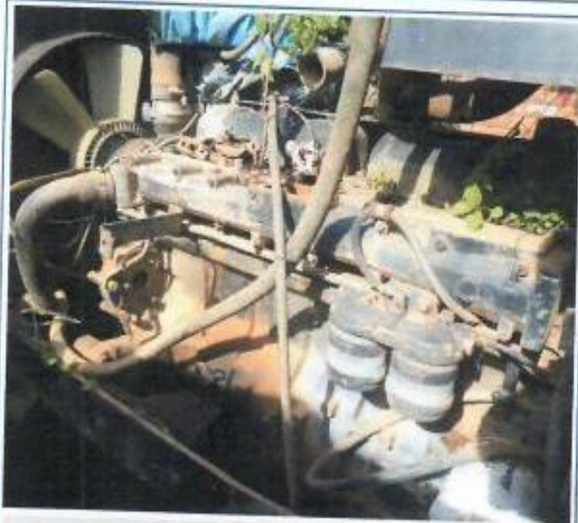
Vista Lateral (Motor de 6 Cilindros TURBO-DIESEL INTERCOOLER)
